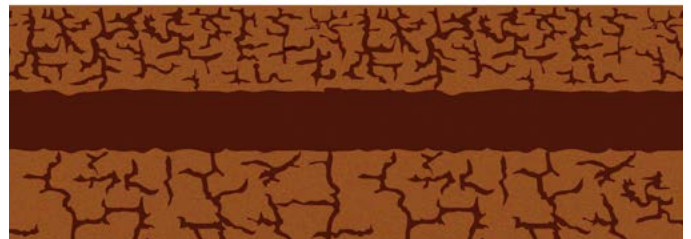
Figure 8. Compaction pans – dense layers caused by farm machinery operation; often 50–100mm thick, they generally have a platy structure and frequently contain crop residues
