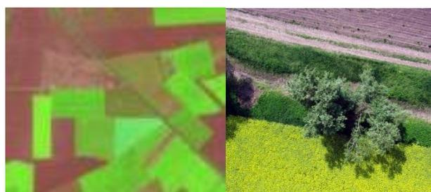
**Fig. 6 Spatial resolution comparison of Satellite (LandSat 7.) and UAV based images**
