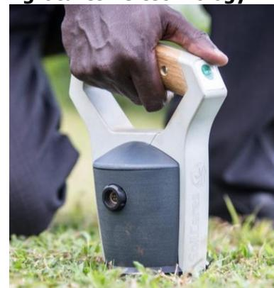
Provides a solution to scan the nutrients in soil, feed or leaf with an easy-to-use handheld tool. Information about the nutrient status on the soil /feed is available on a smartphone within minutes, through a deep learning database and the nutritional database of Trouw Nutrition.
