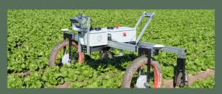
The LightWeeder is a world-first eye-safe, herbicide-free, carbon neutral, commercially viable weeding system delivered by lightweight autonomous field robots via UK agri-robotics company and Agri-EPI Centre member, Earth Rover.
