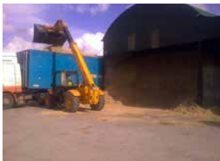
Chipped miscanthus being loaded onto a walking floor trailer ready for delivery to a power station
