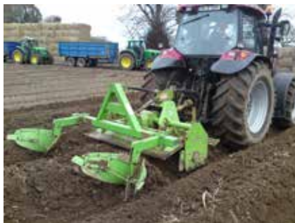
The spike rotavator turns the rhizome
