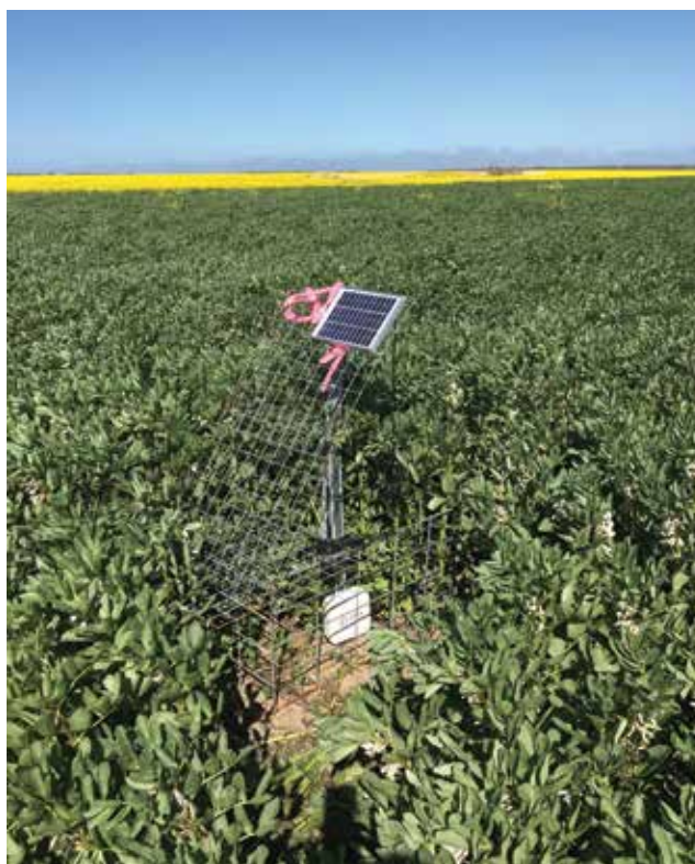
Figure 8.9: A data logger set-up at the Kojaneerup trial logs environmental conditions hourly via the Telstra narrow-band network. The data are available in real-time online, and the system is programmed to send spray alerts via email.
