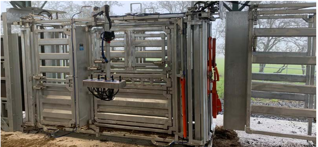
Figure 3. Air-operated crush with fully adjustable sides
