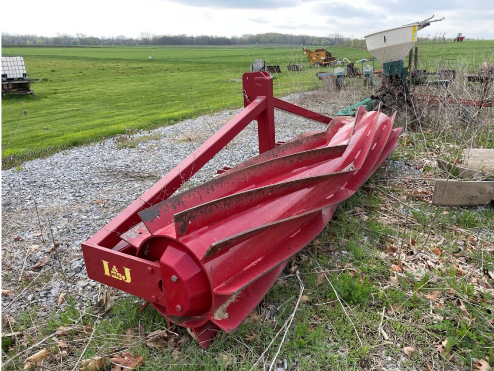
Figure 12 - Crimper roller in New York State used for non-herbicide cover crop termination Source: Author
