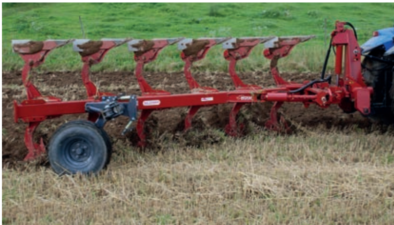
Stubble tillage with a skin plough (Precilab). Only the upper 10 cm are being ploughed. The depth can be adjusted via support wheel. The root weeds are being severed and are lying on the top where they dry out.
