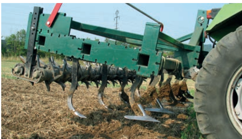
The flat cultivator, undercutting the whole surface, can achieve a similarly efficient result against root weeds as the stubble-plane plough or the skin plough. Unlike the skin- or stubble plane ploughs, it does not turn the soil.
