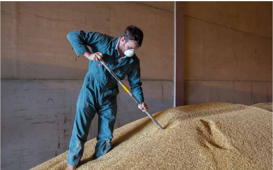
Figure 10. Sampling grain from a heap using a spear
