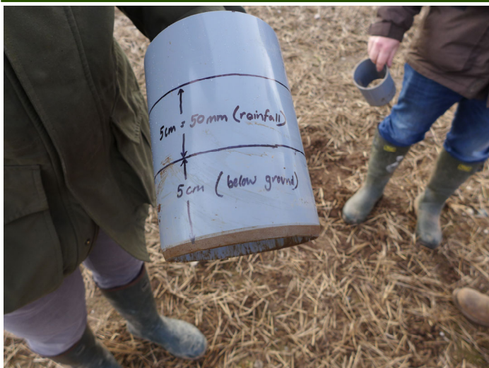
1. Measure and mark lines on pipe
