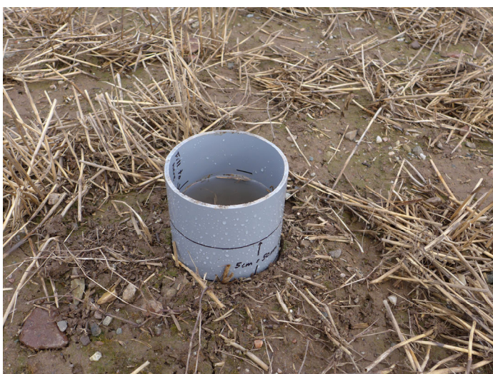
3. Fill with water to the 10 cm line and start timer
