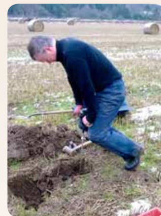
A penetrometer can be used to identify the depth of soil compaction in fields
